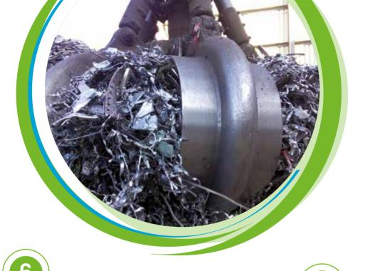
Slag production is much reduced and may be more than halved in comparison with slag from sheared or baled scrap grades, which means savings on additions of slag formers such as lime, leading to a higher productivity.
