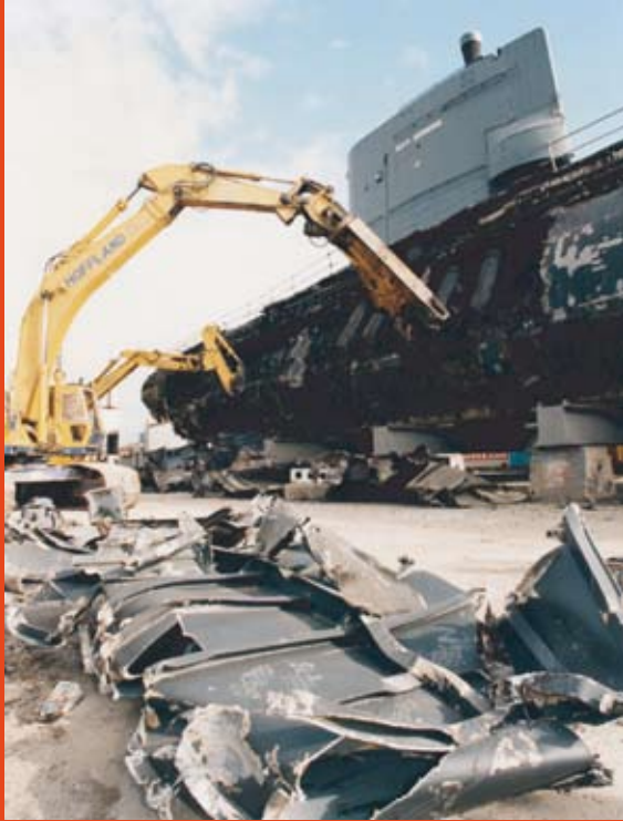
Modern dismantling of a Dutch submarine. With the assistance of two hydraulic excavator scrap shear attachments (LaBounty and Veratech/Verachtert), the dismantling of all kinds of ships has become much faster and cheaper.
