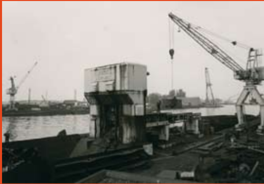
The first hydraulic guillotine shears date from around 1960. This hydraulic Lindemann 'Lusic' shear was installed in 1962; it had a cutting force of 540 tons and, at that time, the machine room was positioned above the cutting head.
