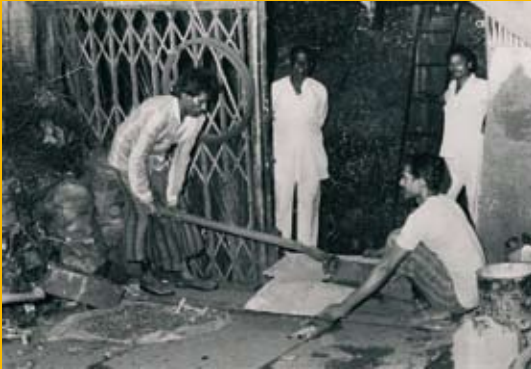
Cutting scrap with a primitive hand-made scrap shear, as was done centuries ago; photo by courtesy of Ikbal Nathani, India.
